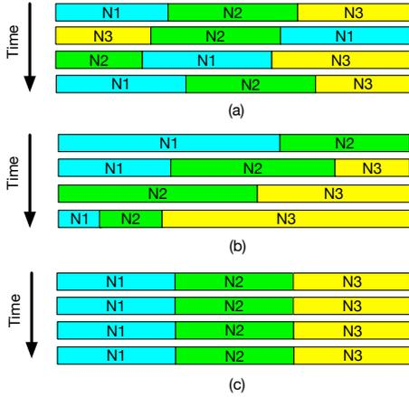
Fig. 2. Resource allocation for 3 numerologies over multiple TTI. (a) Resource allocation for ANRA. (b) Resource allocation for PBNA. (c) Resource allocation for CB.
