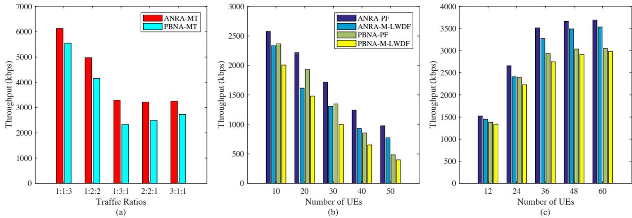
Fig. 4. (a) Simulation A: Aggregate Throughput of Numerology 3 with different traffic ratios using MT. (b) Simulation B: Aggregate Throughput of Numerology 3 under varying number of UEs. (c) Simulation C: Total aggregate cell throughput under varying number of UEs.
